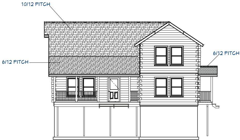
Exterior Elevation Front
